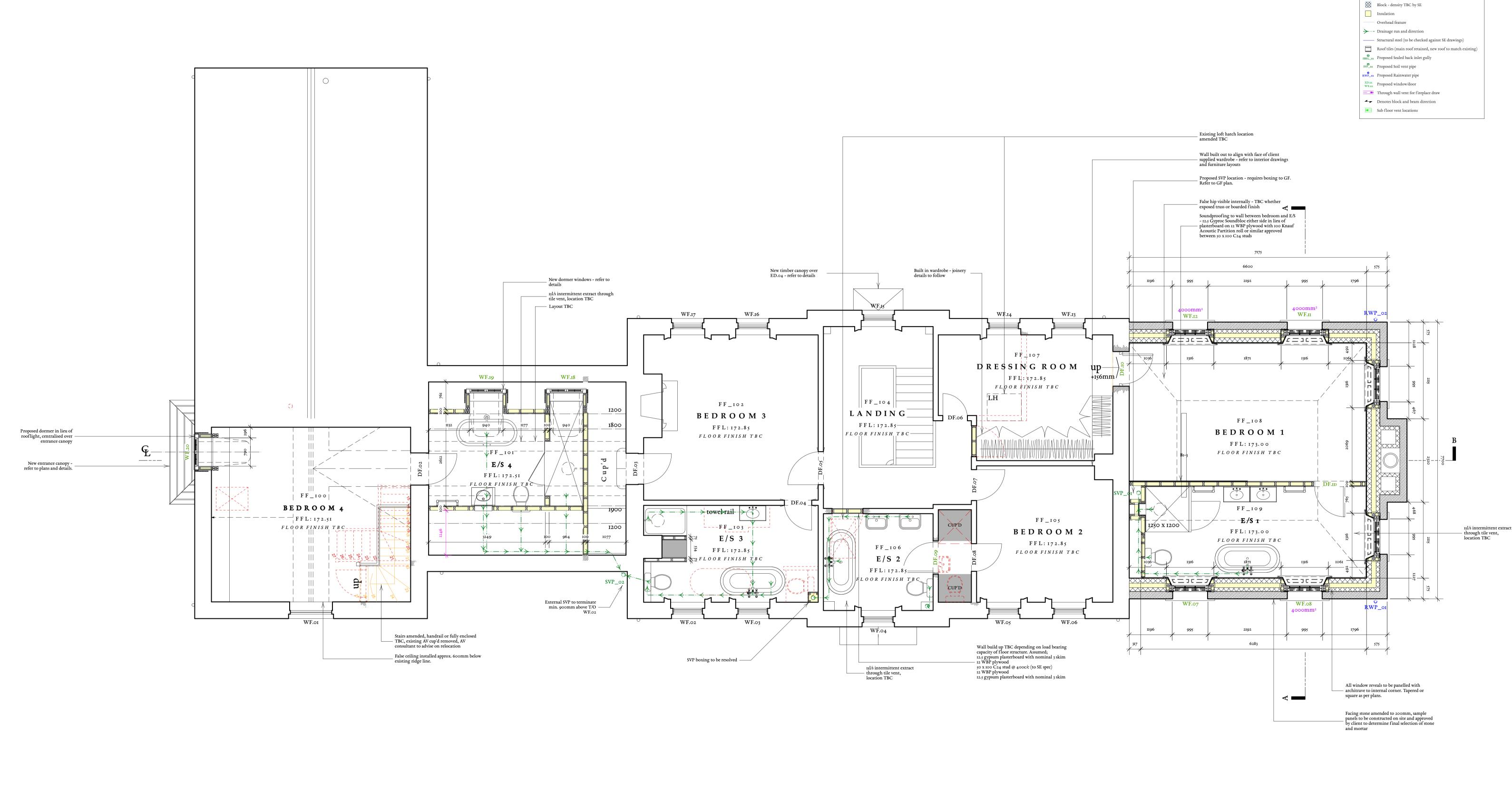
All internal stud work to be 47 x 100 C24 timber @ 400cc, lined to room sides with 12 WBP ply and 15 gypsum based plasterboard, 3 nominal skim finish, fully insulated with Knauf Acoustic partition roll. Gyproc Soundbloc to studs between wetrooms, bedrooms and living spaces.
